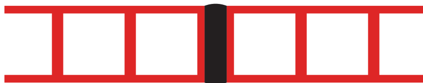
Spirolite Thermal Welded Bell and Spigot Joint
