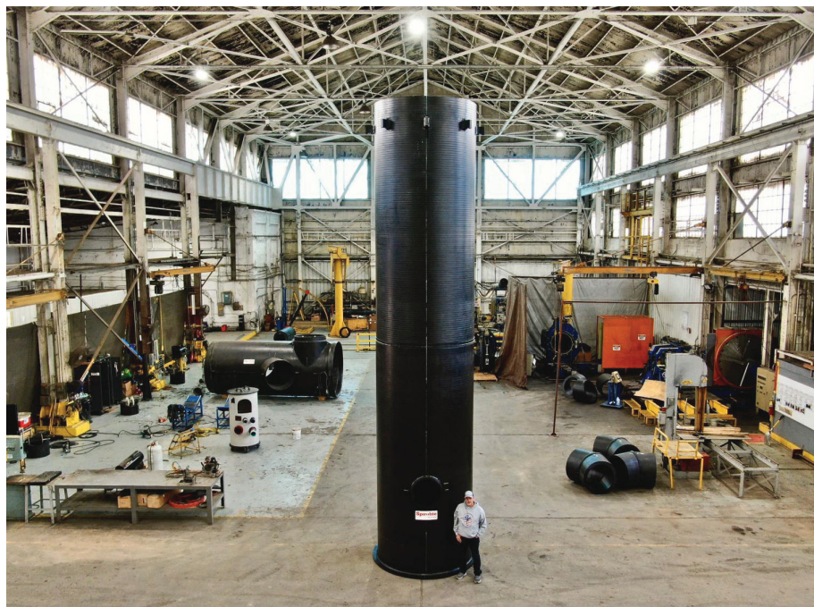
This 31-foot manhole was manufactured from solid-wall Spirolite pipe.
